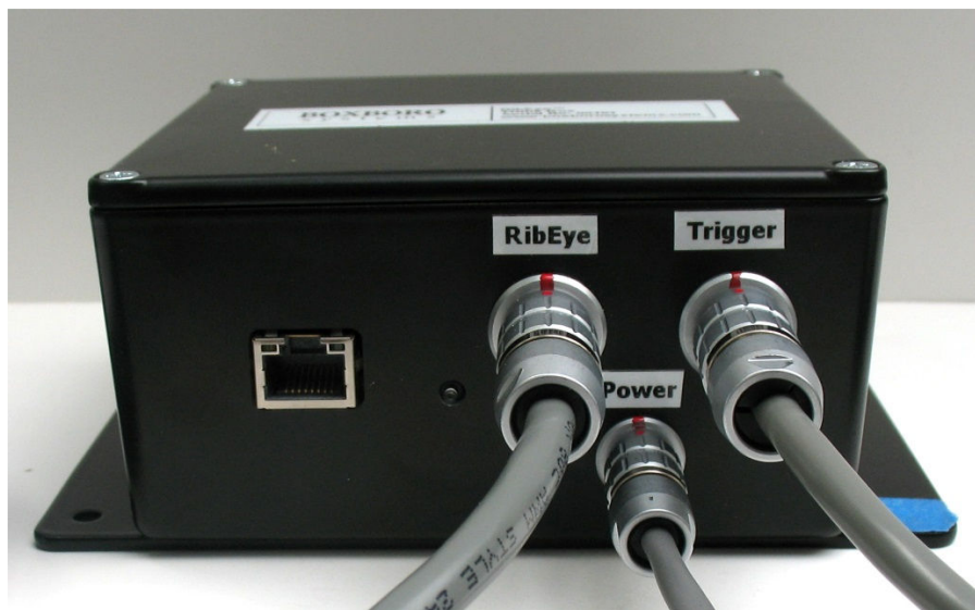
Figure 10. RibEye trunk box for Hybrid III dummies
